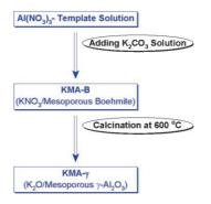
Basically super: Potassium-functionalized mesoporous γ-alumina solid superbases that have a high base strength  $(H_{-})$  of 27.0, a well-expressed mesoporous structure, and which are efficient in the isomerization of 1-hexene are synthesized by a one-pot method. The success of this method can be ascribed to the flexible application of K2CO3 as a pH adjustor and close control of the calcination process (see picture).
