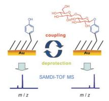
Sugar coated: A new strategy for solidsupport oligosaccharide array synthesis and direct SAMDI-TOF (self-assembled monolayers for matrix-assisted laser desorption-ionization time-of-flight) mass spectrometry detection of the synthesis process is reported (see scheme). It incorporates an on-chip ligand array synthesis, a label-free detection method, and direct application to an enzymatic assay.
