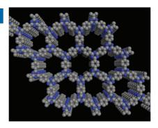
Ordered and amorphous microporous polytriazine networks have been obtained from the trimerization of nitriles in a ZnCl<sub>2</sub> melt at 400 °C (see structure of the polymer formed from 1,4-dicyanobenzene; C gray, N blue). The materials are high-performance polymers with very large surface areas and could find applications in gas storage, as sensors, or catalyst supports.
