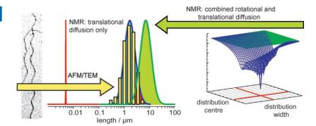
Telling fibrils: Diffusion data obtained by solution NMR spectroscopy from flexible regions of amyloid fibrils for both rotational and translation diffusion combined is of similar magnitude to that measured using AFM and TEM (see picture). Fibrils
