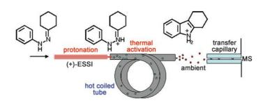
A mild-mannered process: Novel methodology, in which electrosonic spray ionization (ESSI, see schematic diagram) is used as the proton source, has been used to generate ionic reaction intermediates whose conversion into products can be
