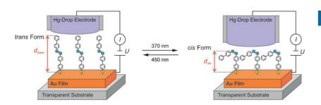
We have liftoff! Tightly packed selfassembled monolayers (SAMs) of ultrarigid conjugated azobenzenes incorporated into a Hg-based junction undergo reversible photoisomerization (see picture). The current-voltage curves indicate that the junction operates as a current photoswitch as result of the forces expressed by the SAMs, which act as a light-powered cargo lifter.
