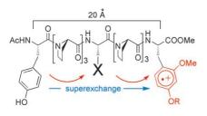
It works both ways: The mechanism of electron transfer through peptides depends upon the side chain X located between the electron donor and the electron acceptor. Electron transfer occurs either by a slow single-step superexchange or by a two-step hopping process that is 20–30-times faster (see scheme). All intermediates in the hopping process could be observed simultaneously.
